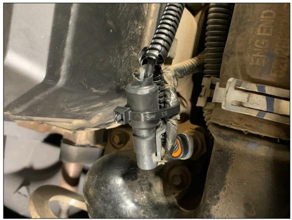
FIGURE 3 – WIRING SECURED AT COOLANT TEMP SENSOR
