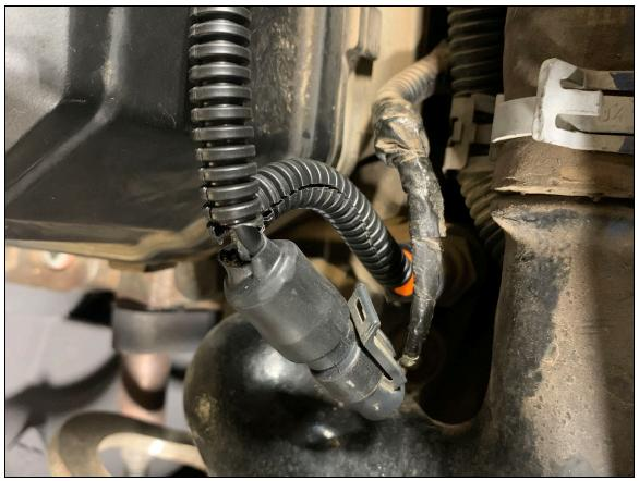
FIGURE 2 - FAN CLUTCH ACCELERATOR INSTALLED
