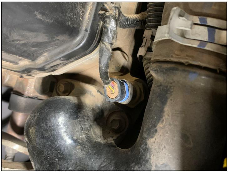
FIGURE 1 – COOLANT TEMPERATURE SENSOR
